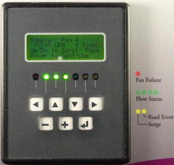
To display information about other fans in the array press the ^ or v keys and the display will scroll through the fans in the array. Each key press will update the fan number and the flow and pressure data on line two. The scrolling function will wrap around the number of fans in the array showing only valid fan numbers.
