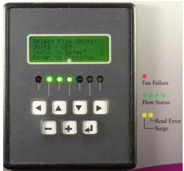
From the “Control Set Up” submenu scroll down to highlight “3. Flow Units”. Press the  $\leftarrow$  (enter) key to display the flow unit set up screen. The first line will read “Select Flow Units”. The second line will read “Units = cfm”. The text after the = sign is the units used to report flow. The last two lines are navigation aids.
