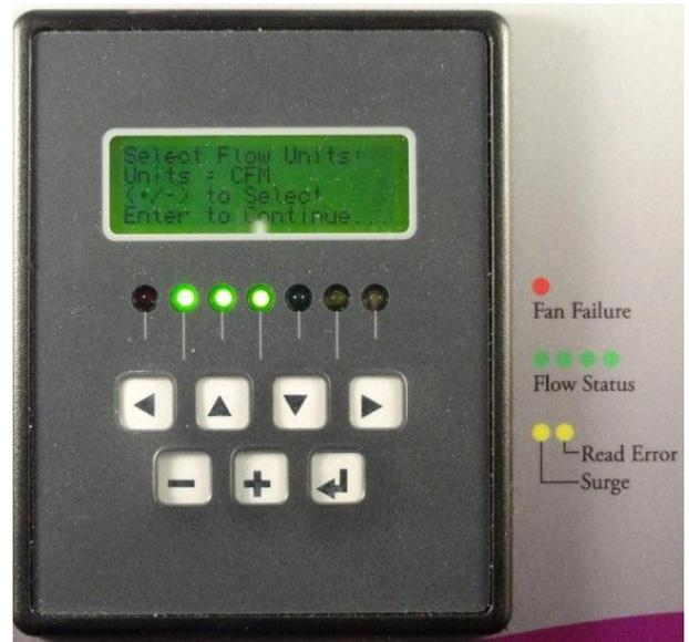
From the “Control Set Up” submenu scroll down to highlight “3. Flow Units”. Press the **↵** (enter) key to display the flow unit set up screen. The first line will read “Select Flow Units”. The second line will read “Units = cfm”. The text after the = sign is the units used to report flow. The last two lines are navigation aids.
