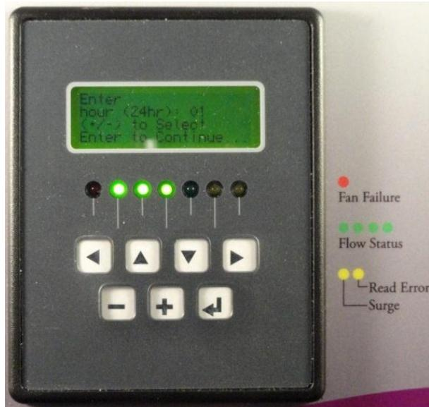
The number after the colon is the minute. To change this to the actual minute press the + key until the current minute is displayed on the first line. It will increment by 1 minute for every key press and auto scroll if the key is held for more than 1 second. If you overshoot the minute you can use the – key to back up. When you have the correct year on the display press the ↵ (enter) key. The following lines will appear on the graphic display:
