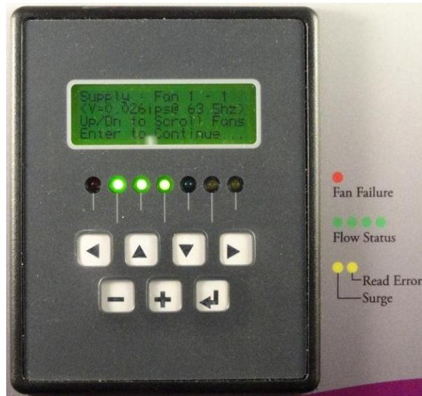
To scroll between fans in the array use the ^ and v keys.
