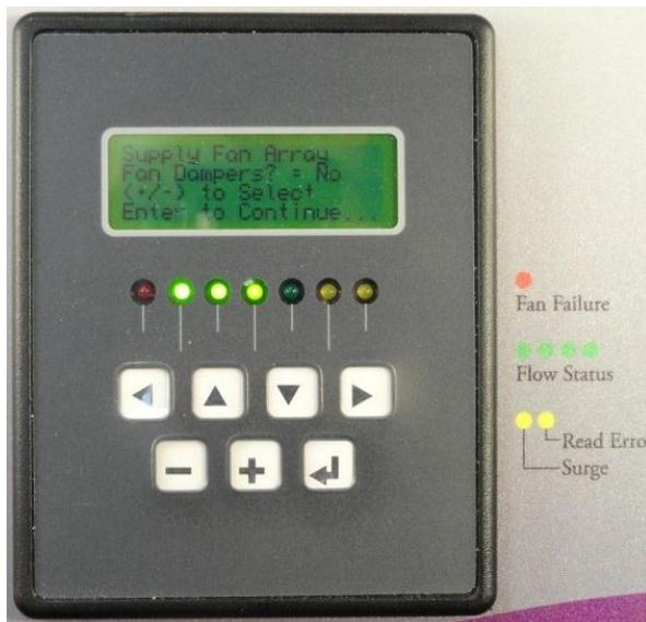
From the "Array 1 Options" submenu, scroll down to highlight "6. Dampers". Press the ↵ (enter) key and the damper setup screen will appear. The first line on the screen will display the array name. It should have been set in a previous step. The second line on the screen will read "Fan Dampers? = No". The description after the = sign is the current selection. The default value is "No". It can be switched between "No" and "Yes"
