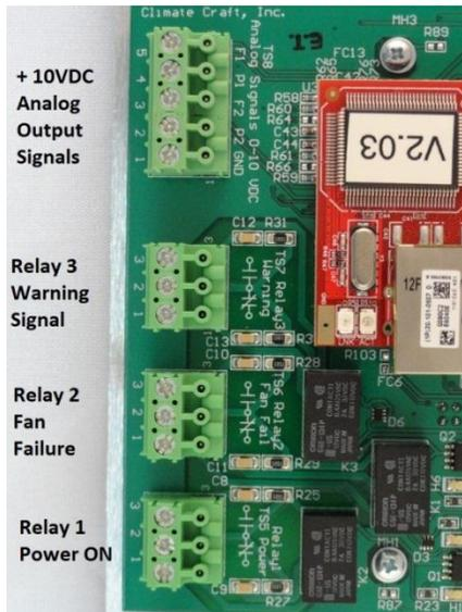
Relay 1 is connected to TS5. It switches when MatrixMonitor™ powers up. It is used to signal the BMS that the control is turned on and available. As long as the control has power and is operating this relay will be switched on.
