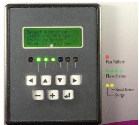
monitored by this unit. The number can be adjusted from 0.100 ips to 0.300 ips in increments of 0.010 ips. The software will wrap around the limits. A “+” key press when the limit = 0.300 ips will result in a limit of 0.100 ips. A “-” key press when the limit = 0.300 ips will result in a limit of 0.100 ips. When the desired vibration alarm limit is selected press the ↵ (enter) key to confirm the selection and return to the sub menu.
