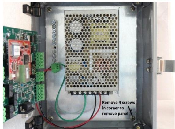
5. Remove all of the connections to the grounding strip.
