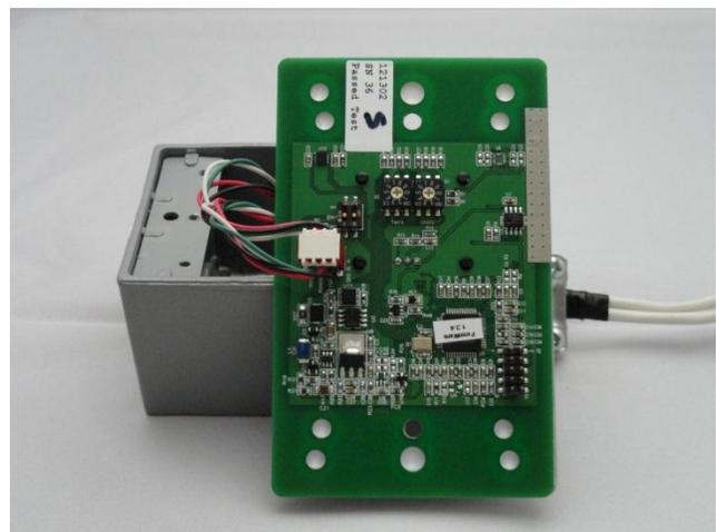
a strain relief cover attached to keep incidental wire movement from pulling on the connection pins which insures a good electrical connection between the cable conductors and the connector.
