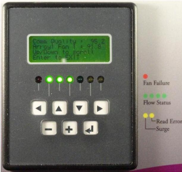
The ^ and v keys allow you to scroll through all of the FSB devices installed on the network. If you press the ^ key the next screen in the sequence will display as follows:
