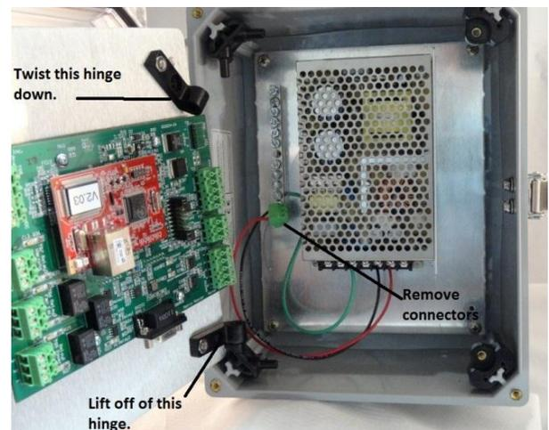
screw from each hinge. The screw to be removed is the inside screw closest to the hinge. There is a lock washer between the machine screw head and the panel. There is a machine nut held in place by a hexagonal cavity on the back of the plastic hinge body. Carefully tap on the hinges to remove these nuts as they will easily fall out once the screw is removed. Store the machine screws, lock washers and nuts for later reinstallation of the panel.
