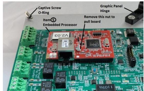
To replace the processor board:
