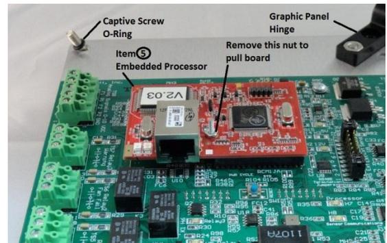
To replace the processor board:
