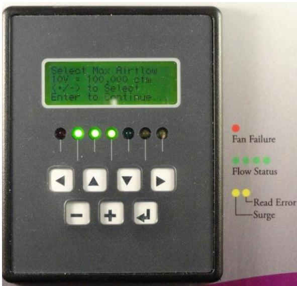
This setting also affects the operation of the green LEDs on the front of the keypad display unit. The green LEDs function as a flow meter for fan array 1. The number of LEDs turned on is controlled by the airflow measured for Array 1 and this setting. The measured airflow of Array 1 is divided by this setting and that result is multiplied by 4 to determine the number of green LED lamps to turn on.
