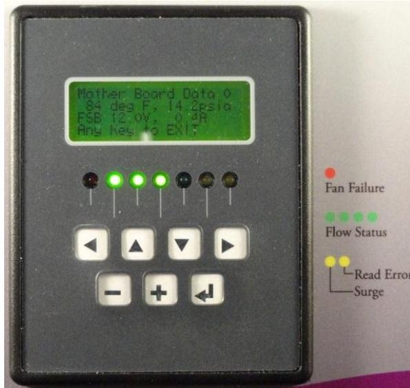
From the “Main Menu”, scroll down to highlight menu selection “12. Mother Board data” and press the ↵ (enter) key. The following will display on the screen:
