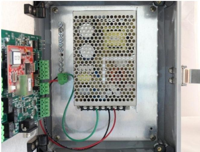
The power supply for the MatrixMonitor™ system is a 100 watt Mean Well Direct model RS-100-12. It is a switching power supply that provides 12 volts DC to the embedded control system, the fan sensor boards and the array pressure rise transducers. It accepts input voltage from 88 VAC to 264VAC at 47 Hz to 63 Hz. The power supply is mounted to the backplane of the control enclosure. The AC supply power connections are made directly to the appropriate terminals on the power supply.
