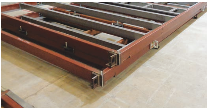
Welded structural base
